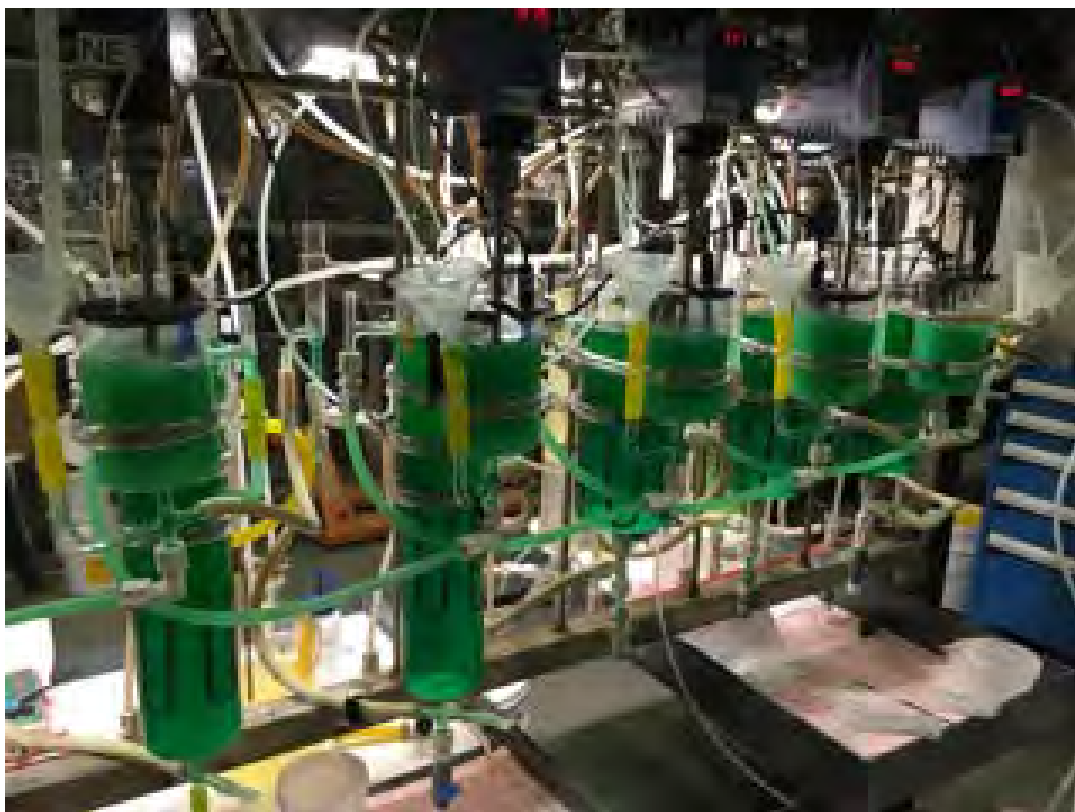
Figure 13-10: Nickel solvent extraction – 5-stage extraction circuit
