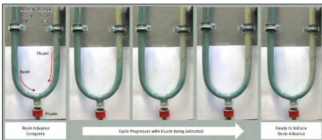
Figure 13-7: U-column desorption front between consecutive resin advances
