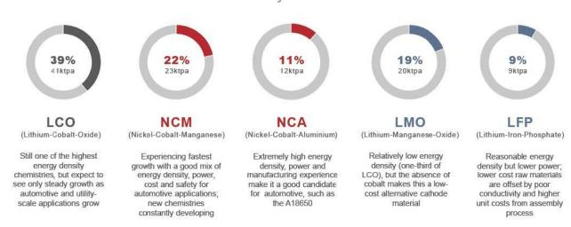
LiB cathode production requires high purity precursor materials to ensure high performance and extended battery life. NCA and NCM battery chemistries require high purity nickel sulphate and cobalt sulphate to produce precursor materials. LCO battery chemistry requires cobalt oxide.
