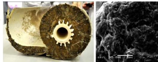
Fouled RO Membrane
